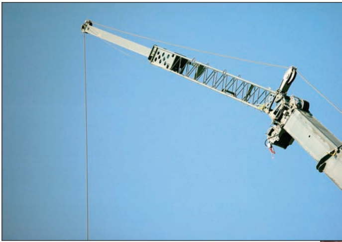
Max. tip height of 154 ft. (47.0 m) w/ 45 ft. (13.7 m) tele. extension
