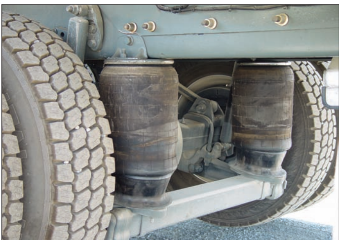
Spring front suspension w/air ride rear suspension provides a comfortable ride at 65 m.p.h. (105 Km/h)
