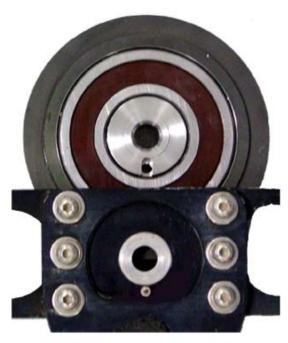
Use a bolt in place of the load pin to hold it in place. Install an allen wrench or other long tool to align the hole in the bearing with the slotted hole in the frame.
