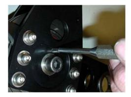
5. Remove the bolt and install the load pin.
