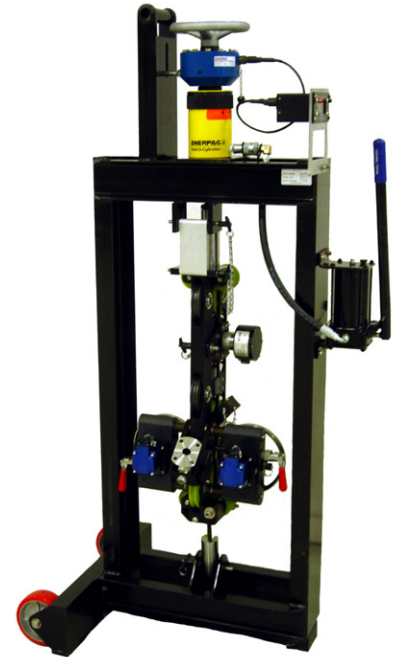
AM5K MEASURING HEAD BEING TESTED ON MODEL 150 SMALL TEST STAND
